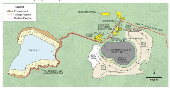
Copper-gold concentrate produced at Pebble is transported via a slurry pipeline to a new deep-water port on Cook Inlet. There it is de-watered and bulk shipped to offshore smelters. Other products of the process plant are gold doré, which would be flown to market from an existing aviation facility at Iliamna, and molybdenum concentrate, which would be bagged and trucked to the port for shipment.
